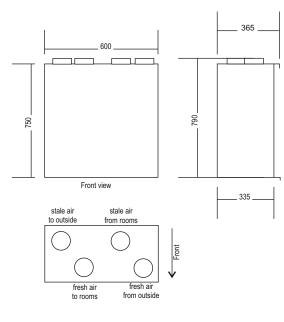
Duct Connections 325-12W= 150mmDuct Connections 200W= 125mm
